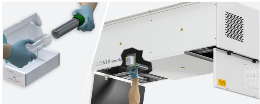
Fig. 27. Take the ionising pipes, remove the bubble wrap and check the integrity of the glass. Gently screw the ionising pipes by gripping them at the base (green part).
