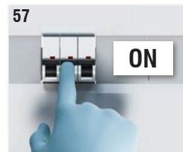
Fig. 57: Act on the safety magnetothermic switch positioned on the circuit upstream of the device to restore the electrical power supply.
